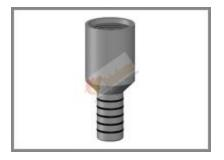
Stab in Stinger allows large diameter casing strings to be cemented through the drill pipe or tubing that is stung into and/or sealed into the float shoe or float collar.
